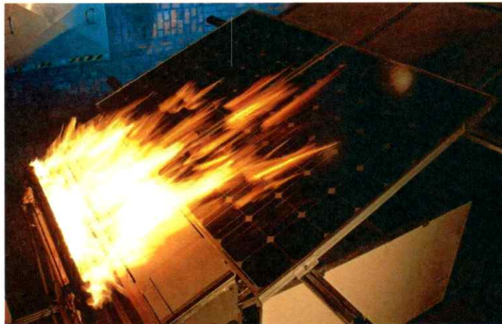
Picture 1: Spread of Flame Test
