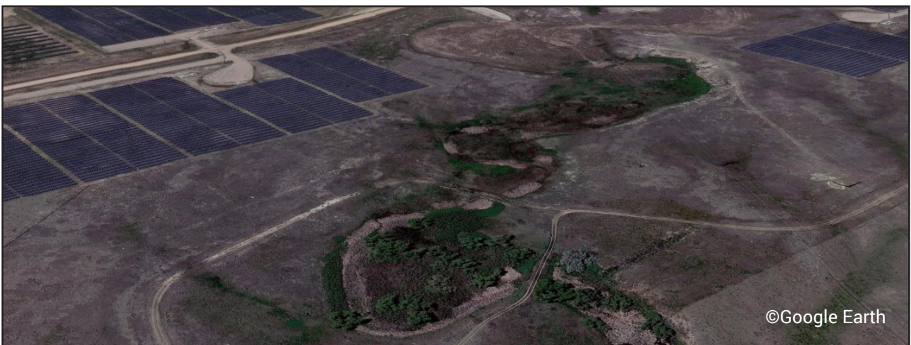
Platte River Power Authority and developers setback the solar facility footprint and fences from this natural drainage to enable wildlife passage and protect water quality, as well as avoid extra development costs and permits.
